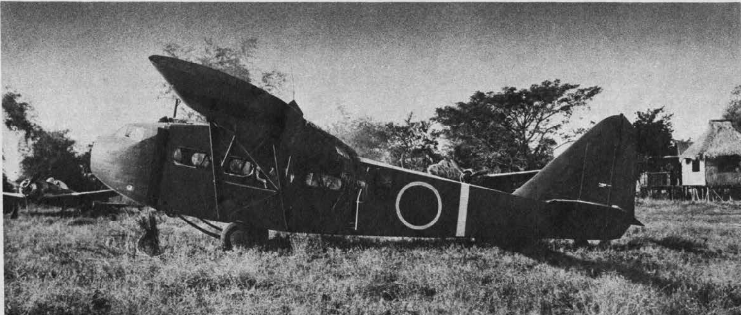
Japanese KU-8 has a tapering fuselage topped off by triangular fin and rudder of conventional Japanese design. The span is approximate-
